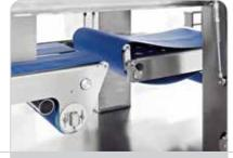
Quick disassembling belt for cleaning
